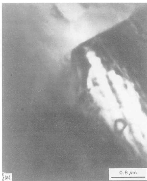
Figure 7 Deformation crossing grain boundary in a rapidly solidified Al-8Fe alloy after isochronal ageing at 500 °C for 2 h, strained under TEM. (a) Crack blocked before the grain boundary; (b) thinning and microvoid formation in the second boundary; (c) opening of the microvoid and joining to the main crack.
